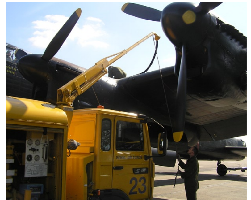
ABOVE With the fuel bowser in position and the boom extended, refuelling begins. (Paul Blackah/ Crown Copyright)
