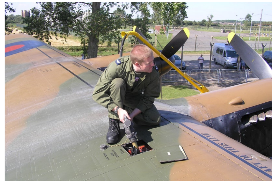
ABOVE With the fuel bowser in position and the boom extended, refuelling begins. (Paul Blackah/ Crown Copyright)
