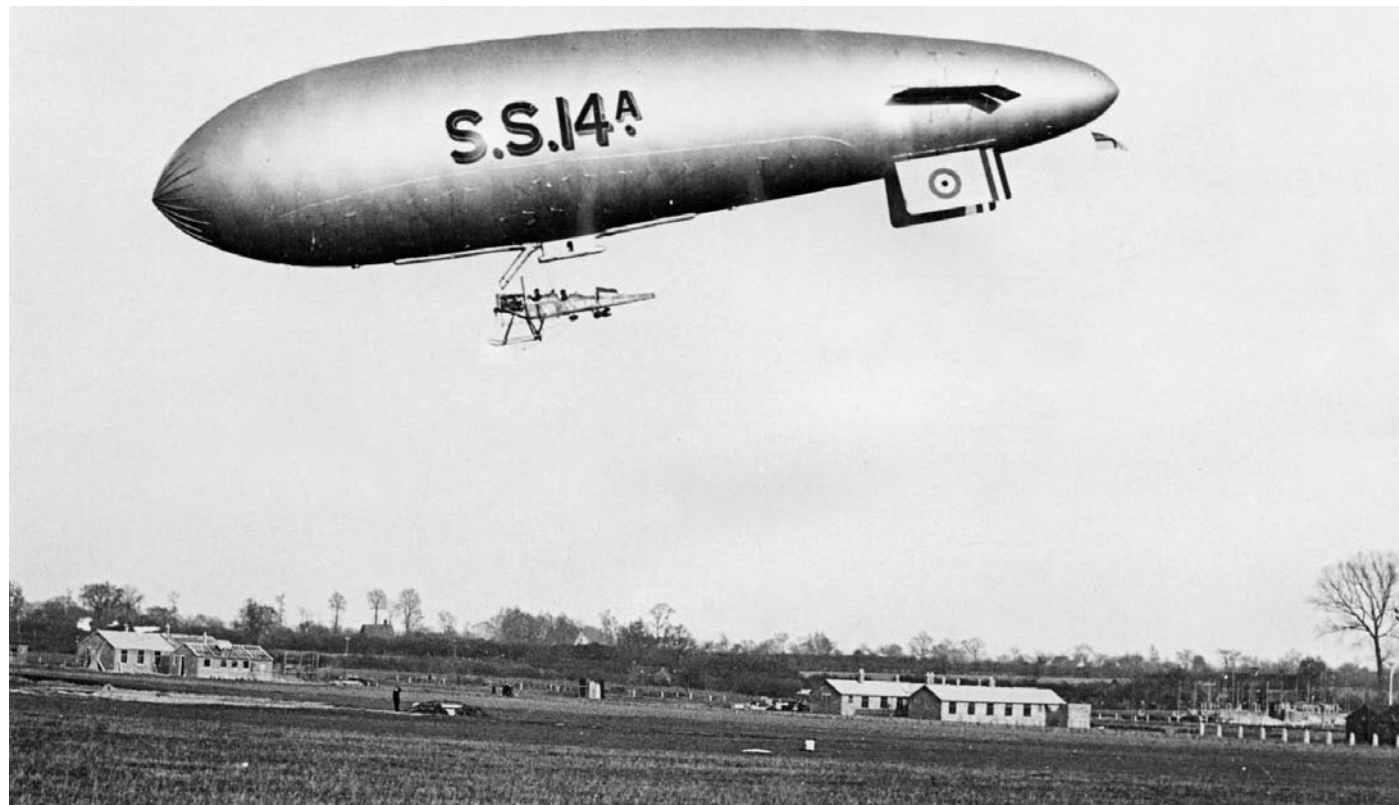
BELOW The SS class of non-rigid airship was developed in just three weeks to meet the new menace of German U-boats late in 1914. These aircraft featured the fuselage and engine of a BE 2C aeroplane hung beneath the gasbag. This is SS 14A.
