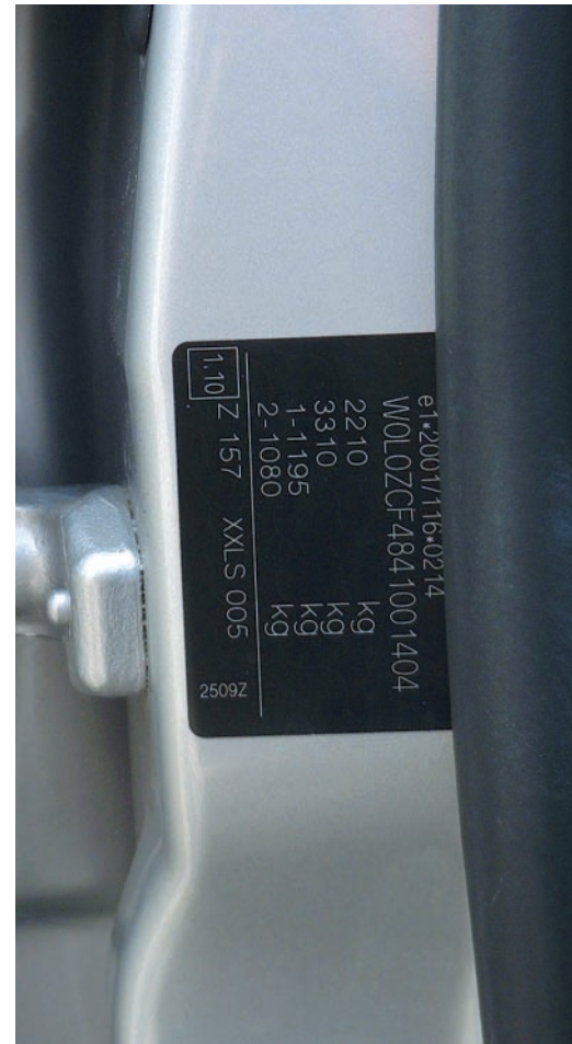
A typical VIN plate, normally found on the engine compartment bulkhead of the car or on the driver's door pillar. The weights show (from the top): maximum permitted mass, gross train weight, maximum front axle load, and maximum rear axle load.
