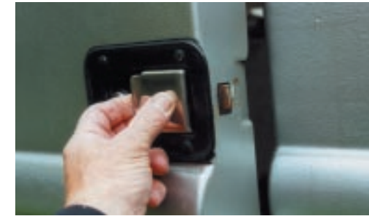
The door catch with its stainless-steel paddle-flap was purchased from Europa, a kit car component supplier.
