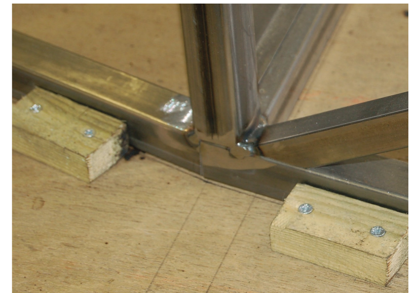
▲ Fig. 4.3 The main bottom rails of the chassis.
