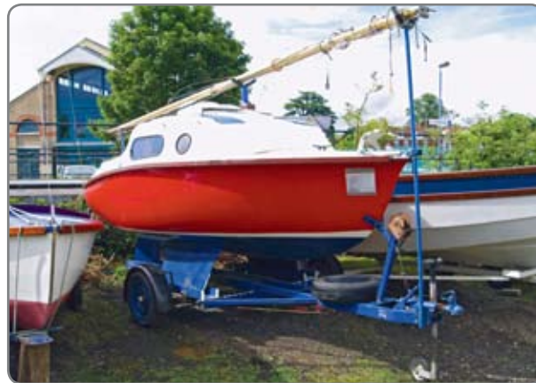
Supports for the mast are provided on this boat's road trailer.
