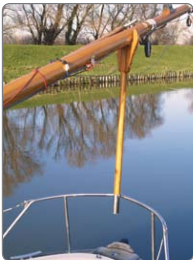
Left: A crutch supports the lowered mast at the stern of this boat.
