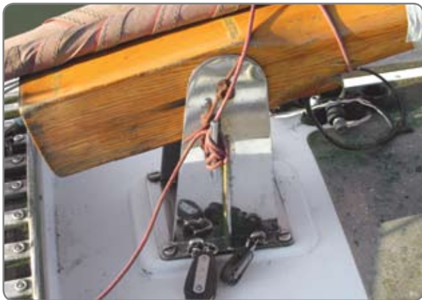
A tabernacle secures the foot of the mast and provides a pivot for mast lowering.
