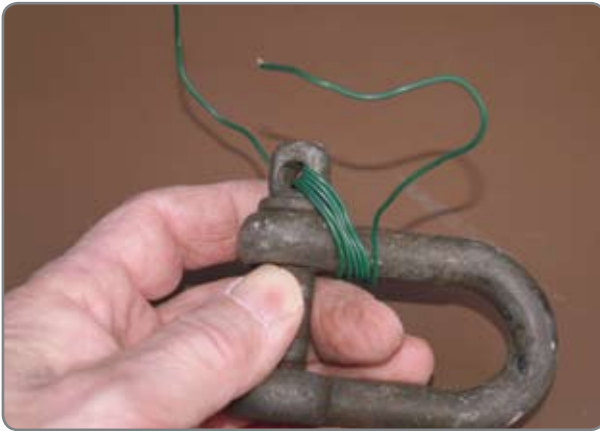
The shackle being 'moused' to stop it unscrewing.
