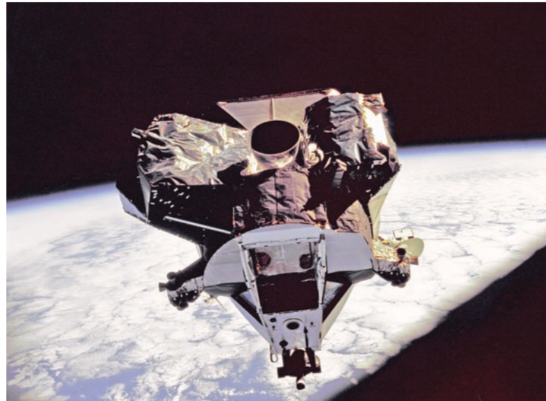
ABOVE The Lunar Module 'Spider' ascent stage is photographed from the Command/Service Module on the fifth day of the Apollo 9 Earth-orbital mission. The Lunar Module's descent stage had already been jettisoned. (NASA)
